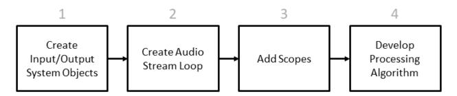
For an overview of the processing loop, consider the completed test bench below. You can recreate this test bench by walking step-by-step through this tutorial.
